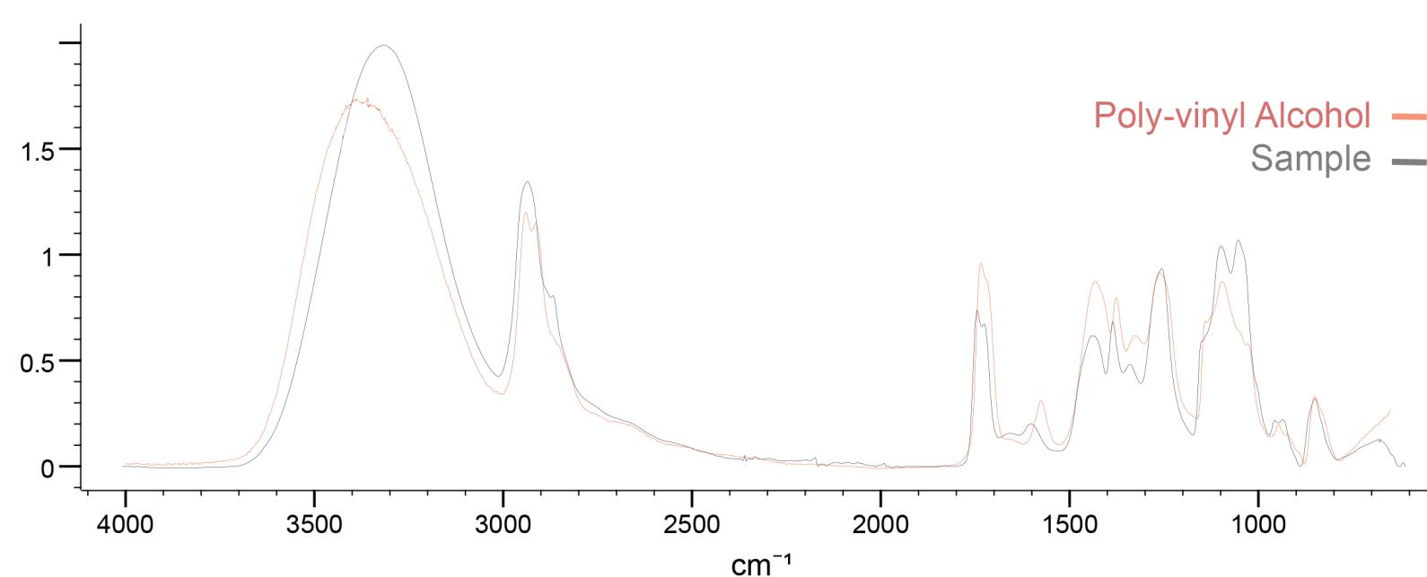
This infrared spectrum analysis shows that the sample of film from the tide pod (black curve) closely matches the spectrum analysis for Polyvinyl Alcohol (red curve), thus confirming that the film on Tide Pods is indeed Polyvinyl Alcohol.
