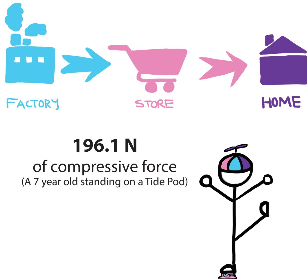
One of the main design considerations for Tide Pods is withstanding forces to prevent popping in transport. We quantified this through impact and compression testing on the Instron. Through our tests, we found that Tide Pods can withstand a surprising amount of force:
